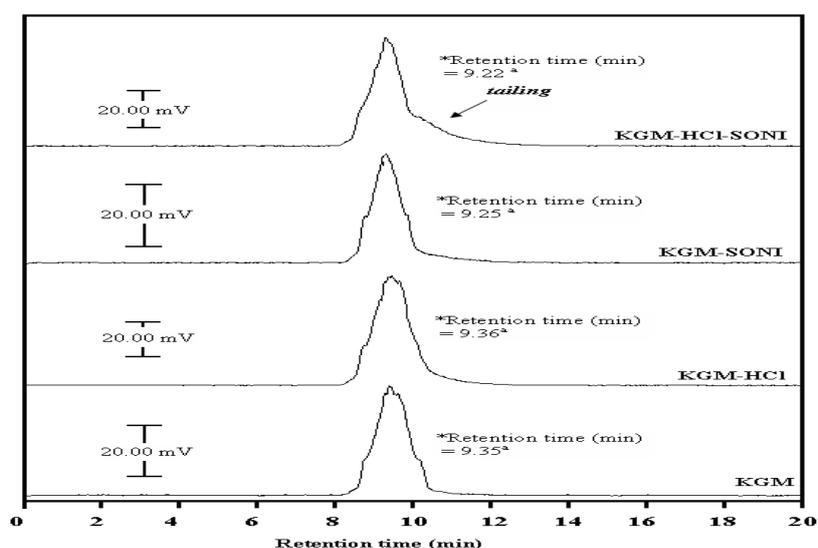
**Figure 2.** Elution profile of control sample (KGM), acid treated sample (KGM-HCl), sonicated sample (KGM-SONI) and ultrasound mediated acid treated sample (KGM-HCl-SONI)
