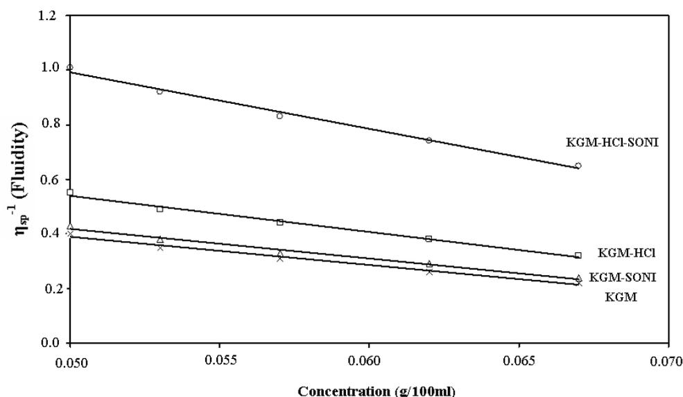
**Figure 3.** Fluidity against concentration for control sample (KGM), acid treated sample (KGM-HCl), sonicated sample (KGM-SONI) and ultrasound mediated acid treated sample (KGM-HCl-SONI)
