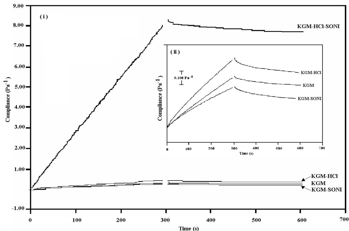
**Figure 4.** Creep-recovery response of (i) of control sample (KGM), acid treated sample (KGM-HCl), sonicated sample (KGM-SONI) and ultrasound mediated acid treated sample (KGM-HCl-SONI); (ii) Inclusion: acid treated sample (KGM-HCl), control sample (KGM) and sonicated sample (KGM-SONI)
